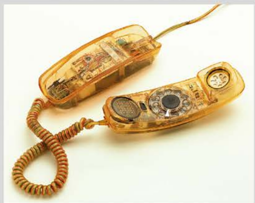
1965 TRIMLINE® This instrument is directed toward the "dial-to-user" concept and is designed as a small combined telephone set with a space-saving rotary dial. It includes a dial light. Service on a national basis followed trial use of different designs produced by Western Electric's model shop in Indianapolis, where the telephone is made.
