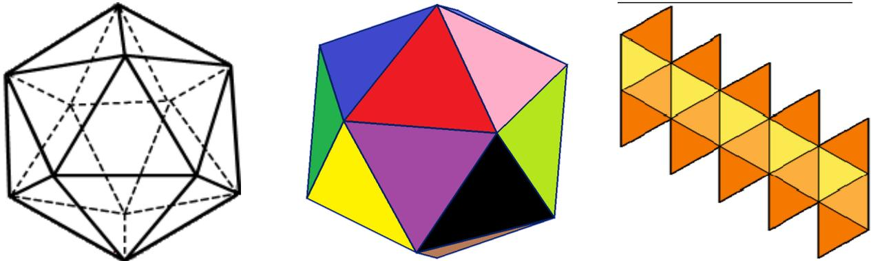
$$R = \frac{a}{2} \sqrt{2+\phi} \quad r = \frac{a}{4 \sin \frac{\pi}{3}} \phi^2 \quad S = 10a^2 \sin \frac{\pi}{3} \quad V = \frac{5}{6} a^3 \phi^2 \quad \theta = 2 \arctg(\phi + 1) \approx 138,19^\circ$$
